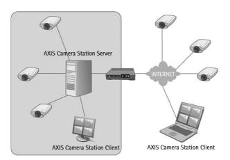
Installation scenario. AXIS Camera Station Server, installed on a dedicated computer, handles the communication with cameras both inside and outside the local (corporate) network. The cameras are monitored and controlled from two AXIS Camera Station Clients — one on the local network and one connected via the Internet.
