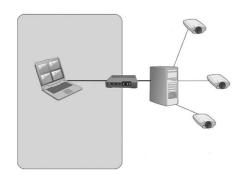
AXIS Camera Station Client behind a proxy. To connect to an AXIS Camera Station Server on the other side of the proxy, the client proxy settings must be configured.
