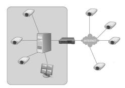
Devices outside of the local network. To access the devices on the other side of the proxy server from AXIS Camera Station, the server proxy settings must be configured.
