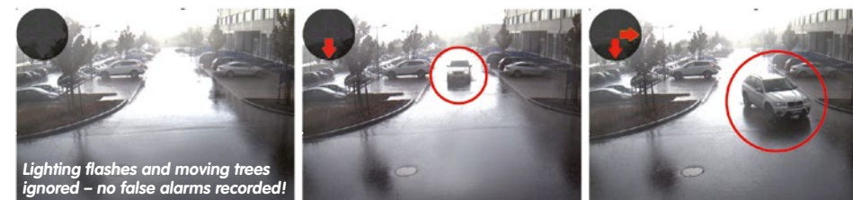
In this sequence, captured by a MOBOTIX camera during a storm, only the moving vehicle is registered, while changes in the scene such as trees swaying, water on the lens and lightning flashes, are all ignored. This world-first in-camera technology can reduce false alarms in cameras located outdoor of more than 90 % .
