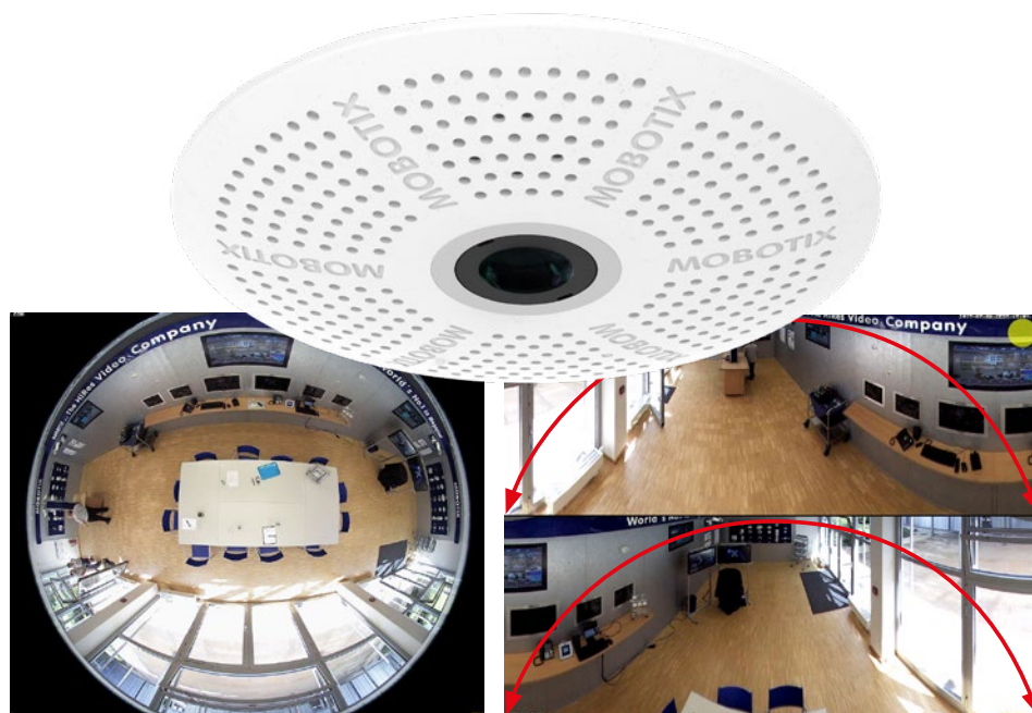
The ceiling-mounted c25 delivers two 180° panorama images of a room.
