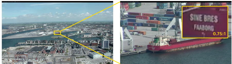
AXIS Q6035-E lets you read texts 1.6 km (1 mile) away. At left, a snapshot of the wide view in HDTV 1080p; at right, 20x optical zoom on a cargo vessel with an inset of the text.
