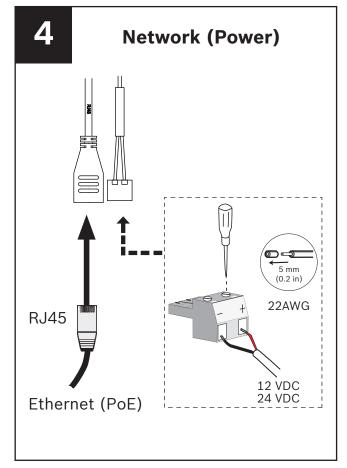
"This product is intended to be supplied by a Listed Power Unit marked "Class 2", "LPS", or "Limited Power Source" and output rated 12Vdc, 0. 32A minimum; or 24Vdc, 0.16A minimum."
