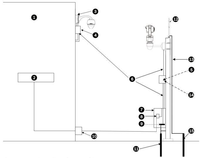
Figure 18.1: Correct outdoor installation with proper surge/lightning protection
