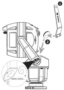
Figure 12.6: Attach the yoke caps.
