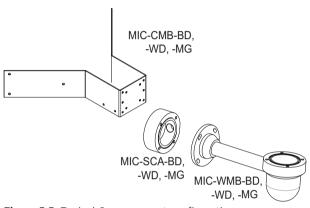
Figure 5.5: Typical Corner mount configuration
