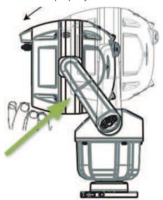
Figure 12.4: Push camera head up 2 mm (0.08 in.)
