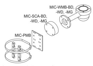
Figure 5.4: Typical Pole mount configuration
