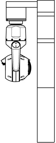
Figure 5.7: MIC camera mounted in inverted orientation (on pole)
