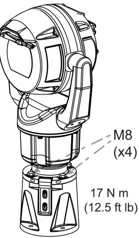
12. Carefully tip the camera to its final position. Avoid pinching wires between the camera base and the DCA! Insert four washers and hex bolts (supplied).
