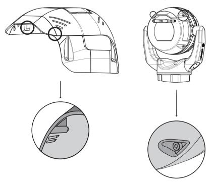
Install the M4 x 10 screws. Tighten the screws to 2.2 N m (19.5 in-lb).
