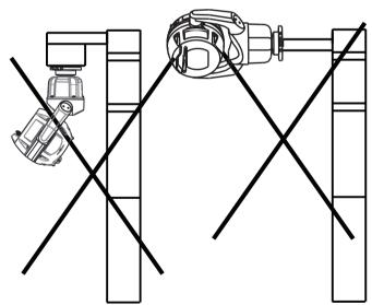
Figure 5.1: Incorrect/not permitted mounting orientations (inverted + canted, horizontal)
