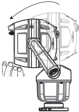
Figure 12.3: Cant the camera head.
