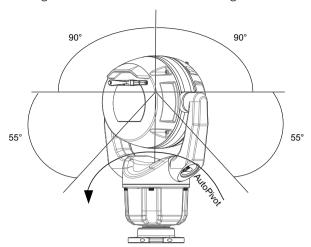
Figure 5.2: Tilt range, MIC IP ultra 7100i
