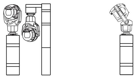
Correct mounting orientation - upright, inverted
