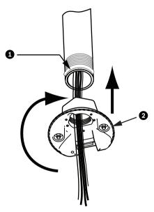
Figure 8.9: Attach Dome Cap
