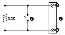
Figure 11.2: N.O.S. - Normally Open Supervised Connections
