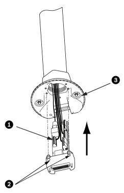
Figure 8.13: Pipe Interface Board to Dome Cap Assembly
