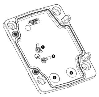
Figure 7.11: Mounting Plate - Inside Detail
