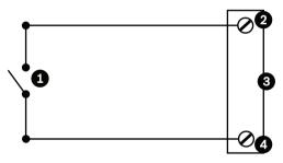
Figure 11.5: N.C. Normally Closed Non-supervised Connections
