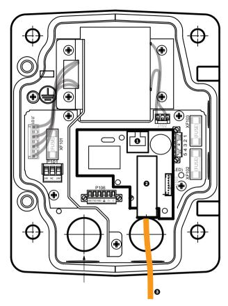
Figure 8.3: Fiber Optic Ethernet Module installed
