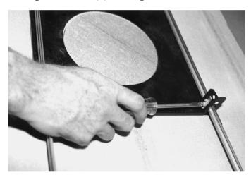
Figure 9.3: Tighten Bracket Securing Screw
