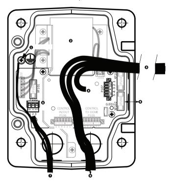
Figure 8.4: Power Supply Box Connections
