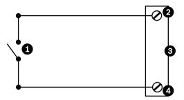
Figure 11.4: N.O. - Normally Open Non-supervised Connections
