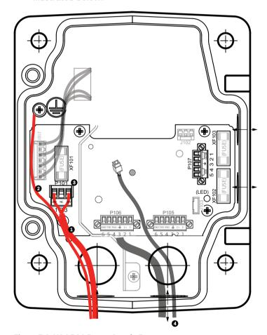
Figure 7.6: VG4-PA0 Power Supply Box
