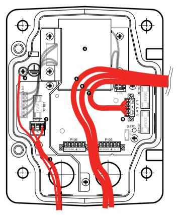
Figure 8.1: VG4-A-PSU1 or VG4-A-PSU2 Power Supply Box
