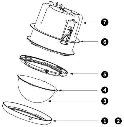
Figure 9.8: In-ceiling (IP54 Rating) Installation Diagram
