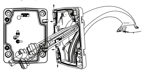
Figure 7.9: Connect Pendant Arm to Mounting Plate
