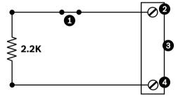
Figure 11.3: N.C.S. - Normally Closed Supervised Connections
