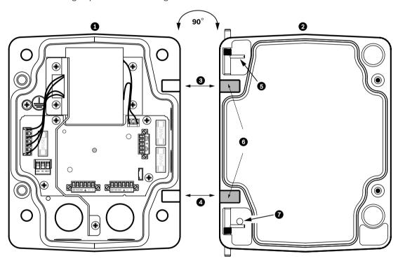
Figure 8.5: Align Cover Door Hinge to Power Box
