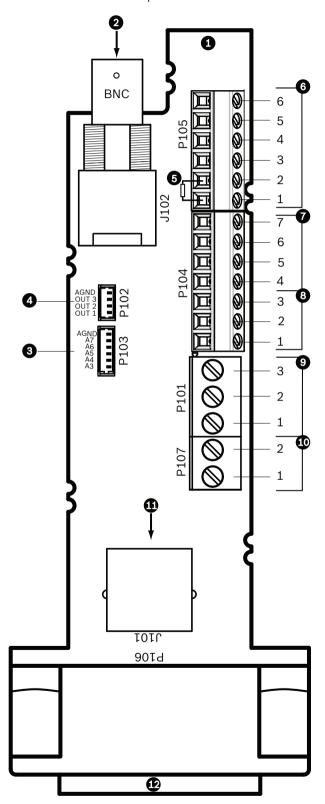
Figure 8.11: Pipe Interface Board Connections
