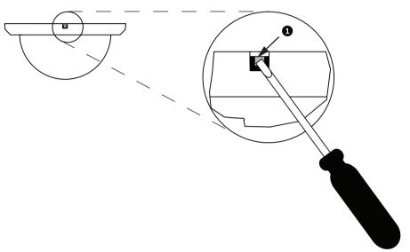
Figure 10.1: Bubble Release Screw
