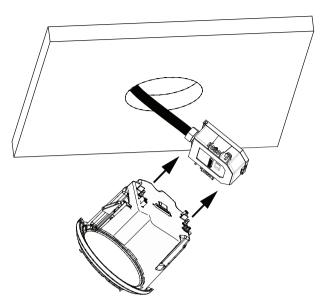
Figure 9.9: Attach Housing to Interface Box
