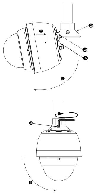
Figure 8.14: Pendant to Roof / Pipe Mount Attachment
