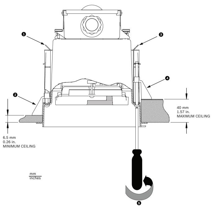
Figure 9.11: Secure camera to ceiling
