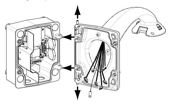
Figure 7.7: Pendant Arm to Power Box Hinge Alignment
