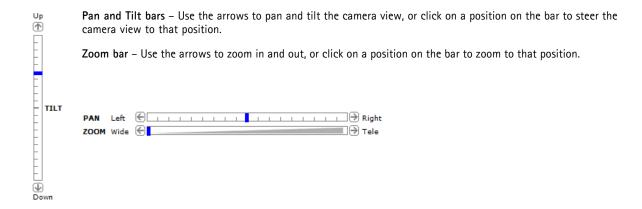
The PTZ controls can be disabled under PTZ > Advanced > Controls, see Controls, on page 26.
